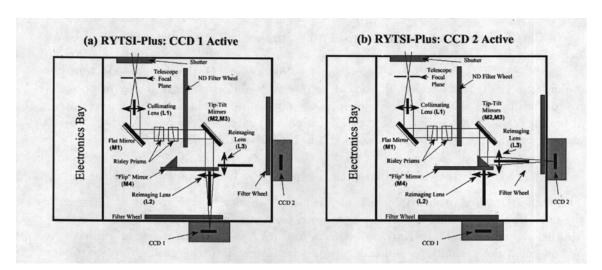
Figure 1: RYTSI-Plus Block Diagram (courtesy E. Horch)
